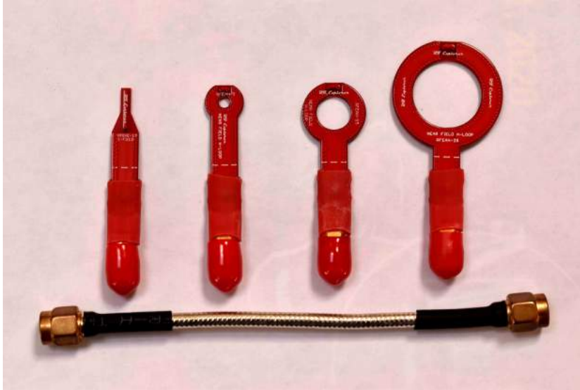
Figure 2.6: Near field antennas of varying diameters and lengths along with a semi-rigid RF cable.
