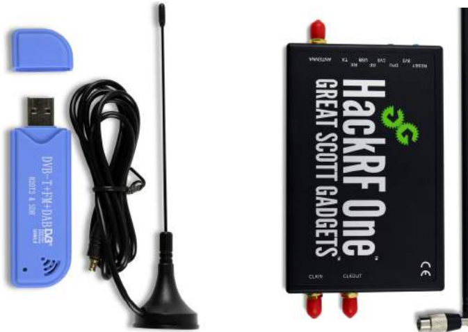
Figure 2.5: RTL-SDR and HackRF One devices with their default antennas.
